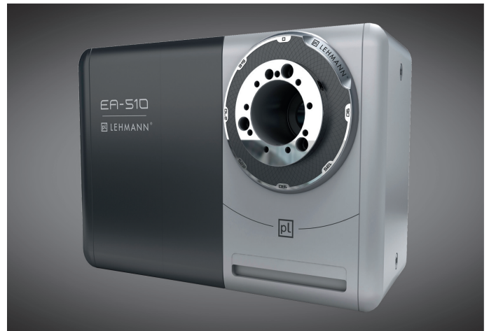
4° axe – 4 te Achse – 4 th axis (Lehmann EA-510, HSK A63)
