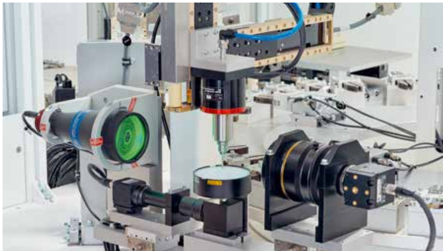
Optical measurement for diameters, lengths, heights, distances, angles, radii and contours
