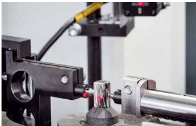
Tactile measuring station for pinions (pitch diameter)
