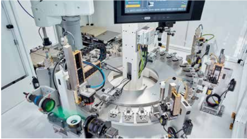
Rotary indexing table with several measuring and testing operation
