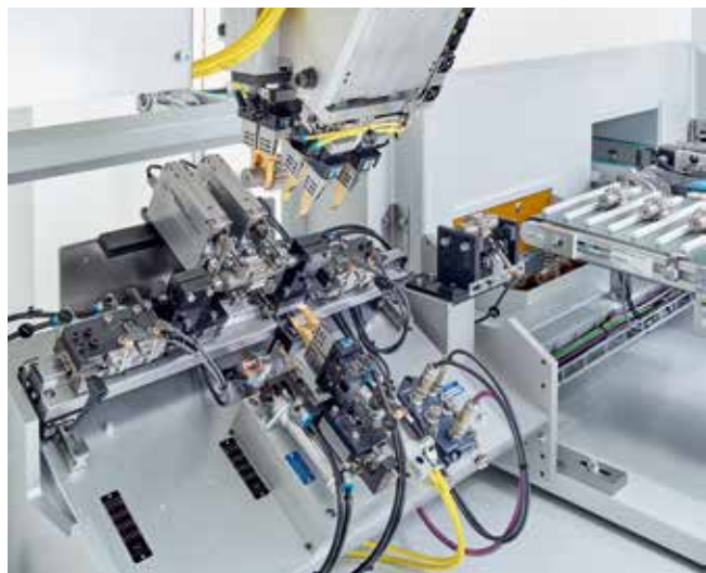
Tactile measuring station for external diameter
