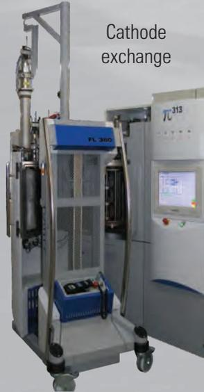
Fork lift for easy transportation of loaded carousels and cathodes to and from the coating unit. Compatible with the machines of the  $\pi$  series.
