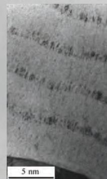
**Nanolayer** is the conventional structure for the so called Nanocoatings. It is a finer version of multilayers with a period of < 20 nm. Typical coating: CrTiN<sup>2</sup>
