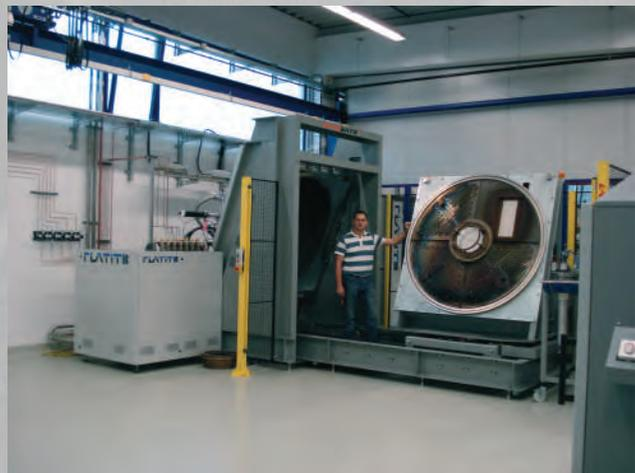
Saw band coils up to 1.4 m diameter can be coated. The back side of the saw band is deposited with a help of a planar target.
