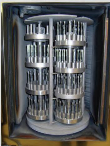
Coating of punches with DLC<sup>2</sup> in the  $\pi$ 111
