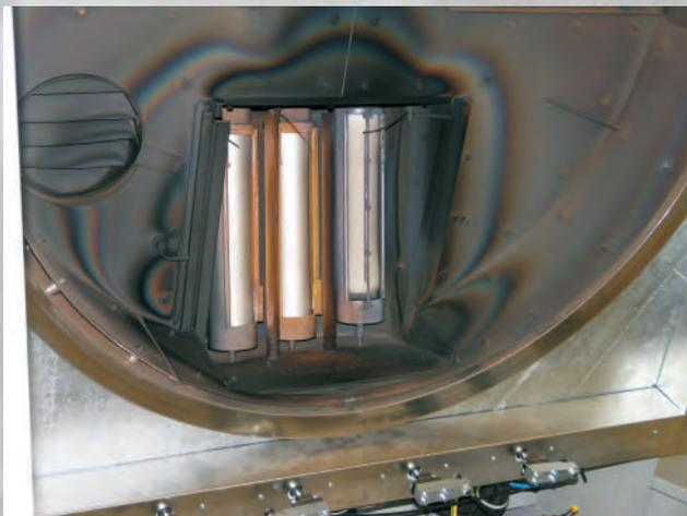
Three rotating cathodes for flexible deposition
