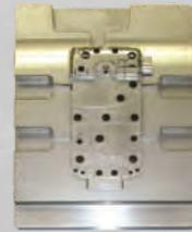
Injection mold coated with nACVlc<sup>®</sup>
