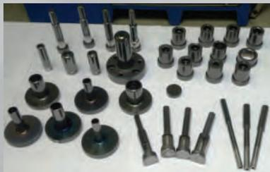
Coated tools for extrusion of aluminum-parts
