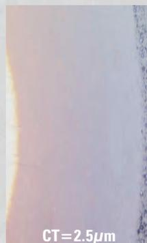
At **gradient structure** the ratio of components (e.g. C) will continuously be changed. Typical coating: TiAlCN<sup>2</sup>
