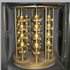
Coating of milling head holders with CrTiN<sup>2</sup> & golden top color by the  $\pi\text{-}303$  configuration.
