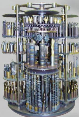
With easy loading, different tool types and sizes can be mixed and coated in one batch.
