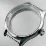
Precision cutting of 3 mm profiles, stainless steel 904L
